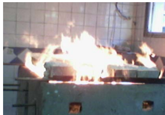
Figure (4): Beams subjected to 650°C (4 hours)
