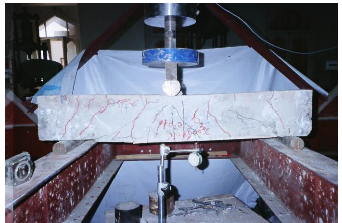
Figure (10): Testing of beam subjected to 650°C (4 hours)
