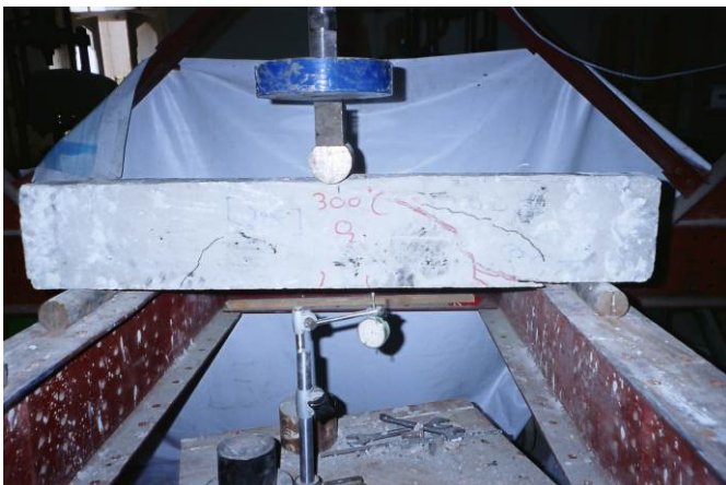
Figure (9): Testing of beam subjected to 300°C (2 hours)
