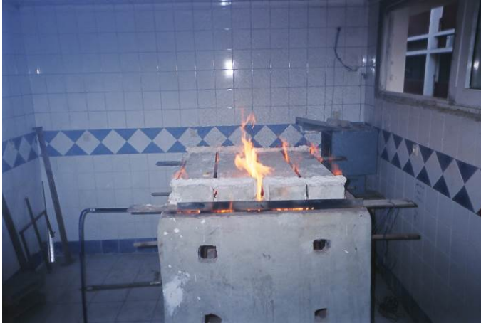
Figure (5): Beams subjected to 300°C (2 hours)
